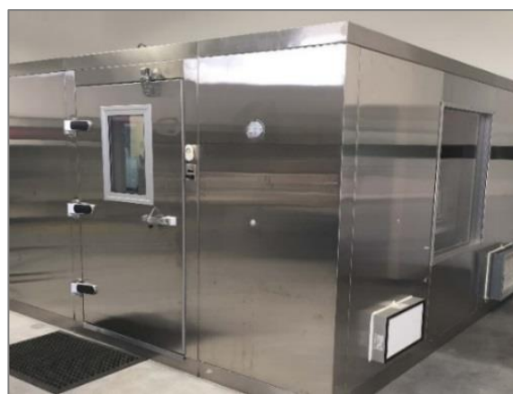
Figure 2: Stainless Steel Bioaerosol Test Chamber used for all M40 Testing. Chamber is equipped with HEPA in/out, multiple bioaerosol sampling ports, decontamination and pressure balance. Exterior picture.
