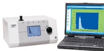
Figure 6. TSI Aerodynamic Particle Sizer (APS) model 3321 used to measure total particle concentration and particle size distribution of the challenge bioaerosol. Range 0.54-20.0 \mu\text{m} aerodynamic diameter, with 1 particle/L detection limits.
